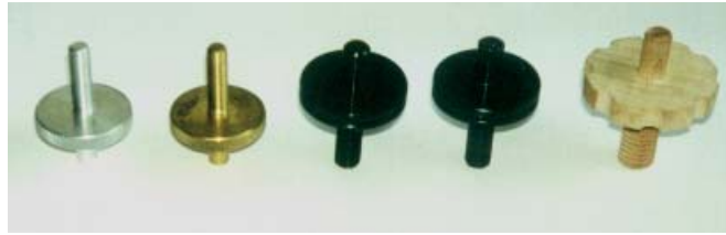
Fig. 4 Aluminum standard, brass standard, aluminum Boehm, polyamide Boehm and maple DiLeone models (lignum vitae Kolstein not shown)
