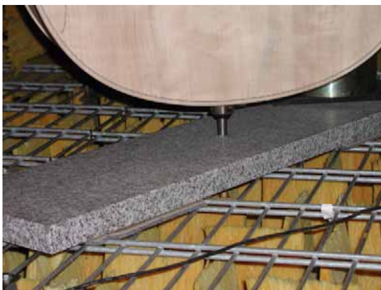
Fig. 5.5. Close-up of artificial endpin on the wire floor of the anechoic chamber
