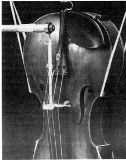
Fig. 3.6. Marshall's set-up, using an impulse hammer applied vertically to the bridge and an accelerometer above the bass bar (Marshall, 1985, 697)
