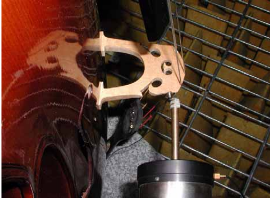
Fig. 5.10. Close-up view of the B&K accelerometer, mounted just next to the needle tip of the shaker. The instrument is the flat-backed cello, Fbc.
