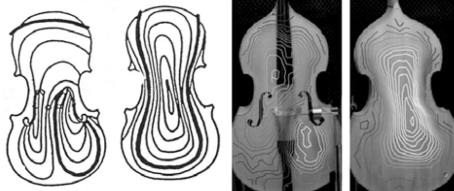
Fig. 6.9. Comparison of C3 mode, 219 Hz (Bynum and Rossing, 1997) and Prb, 155 Hz.
